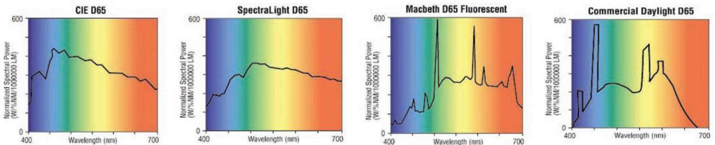
It should be obvious from these SPD curves that the closest simulation to the CIE D65 standard is the SpectraLight D65. The SpectraLight provides daylight using proprietary glass filters, an elaborate power system and specially selected Tungsten Halogen lamps to provide an extremely accurate daylight simulation.
